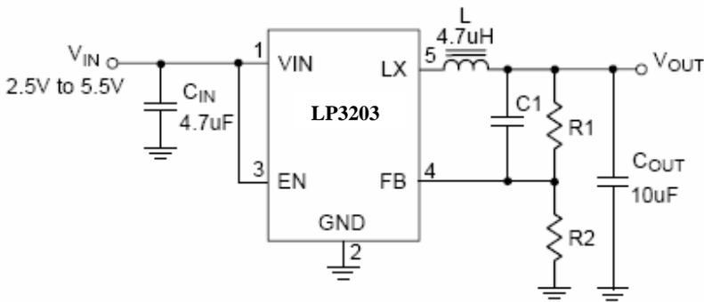
$$V_{OUT} = V_{REF} \times \left( 1 + \frac{R1}{R2} \right)$$
