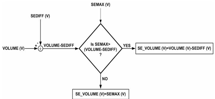
Figure 26. Block diagram of SE Volume Control
