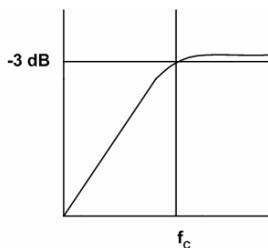
The main disadvantage, from a performance standpoint, is the load impedances are typically small, which drives the low-frequency corner higher, degrading the bass response. Large values of C<sub>C</sub> are required to pass low frequencies into the load. Consider the example where a C<sub>C</sub> of 330µF is chosen and loads vary from 3Ω, 4Ω, 8Ω, 32Ω, 10kΩ, to 47kΩ. Table 2 summarizes the frequency response characteristics of each configuration.
