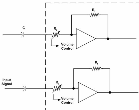
Figure 38. Input Resistor
