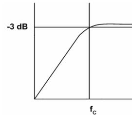
The value of C<sub>i</sub> is important to consider as it directly affects the bass (low frequency) performance of the circuit. Consider the example where Z<sub>i</sub> is 710kΩ and the specification calls for a flat bass response down to 40Hz. Equation 2 is reconfigured as equation 3.
